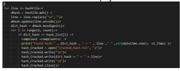
Fig 2.3 main Wordlist function for C++, this reads in all passwords to a memory buffer, removes the new line character and calculates the hash. It then compares the calculated hash with the user hash list provided. if hash match is found it will display the match to the screen and write it to a file
