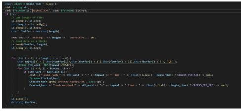
Fig 2.4 main Bruteforce function in C++, this generates all possible four character passwords. Each password is hashed in turn and compared to the user hash list provided. if hash match is found it will display the match to the screen and write it to a file
